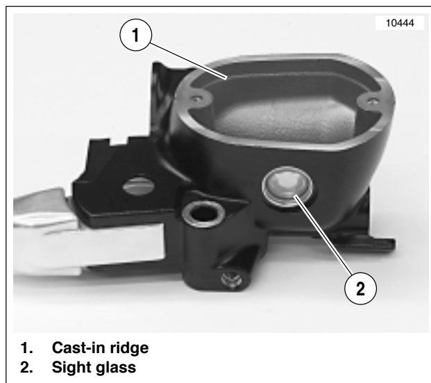
Figure 1-23. Filling Front Master Cylinder Reservoir
