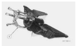
**3.** Use tooling (A) to loosen the flange to the drive shaft. Remove tooling (A), the bolt, washer and flange from the drive shaft.
