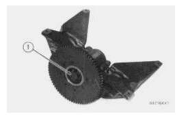
**1.** Loosen bolt (1). Do not remove the bolt at this time.
