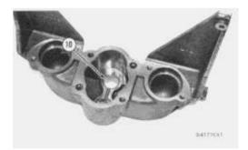
7. If necessary, remove bearings (10) from the pump body.
