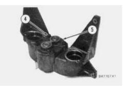
**4.** Put alignment marks on the pump body and cover (5) for correct assembly. Remove bolts (4) to remove cover (5) from the pump body.
