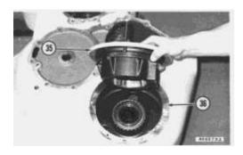
27. Remove bearing cage assembly (35) and shims (36) from housing.
