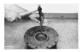
**33.** Use a hammer and a punch to remove the bearing race (44) from the cage.
