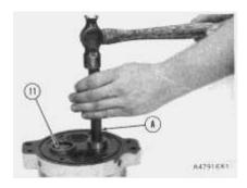
**8.** Remove two bearings (11) from bottom cover with tooling (A).
