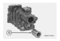
i) Remove retainer (13) from valve body.
