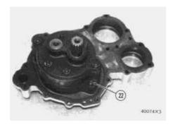
19. Remove the bolts (22) that hold the transmission pump to manifold cover.
