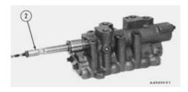
**b)** Remove valve spool (2) from valve body.
