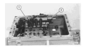
1. Remove six bolts (1). Remove priority valve (2).
