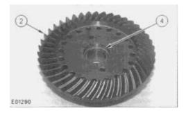
28. Install thrust washer (4) in bevel gear (2). Lubricate the thrust washer face with clean axle oil.
