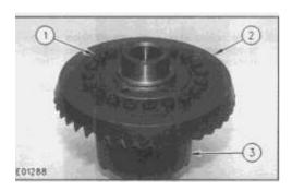
**29.** Invert bevel gear (2) and install on case housing (3).
