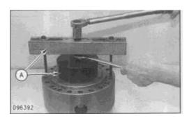
**b.** Tighten the center bolt of Tooling (A) to a torque of 27 N·m (20 lb ft) to apply 900 kg (2000 lb) of preload on the disc packs.
