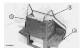
**9.** Remove two bolts and lockwashers (11). Remove two nuts, lockwashers and screws (12). Remove grab iron (10).
