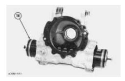
12. Use a hoist or two persons. Remove rack assembly (14). Weight is 80 lb. (36 kg).
