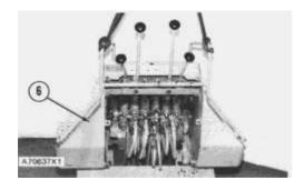
7. Fasten a hoist to the console. Weight is 184 lb. (83 kg). Put console (6) in position on the backhoe. Install the four lockwashers and bolts that hold the console in position.
