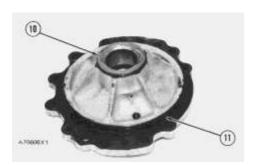
**9.** Remove O-ring seal (11) from the cover. Remove bearing (10) if necessary.
