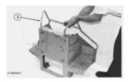
**4.** Put grab iron (3) in position. Install the two screws, lockwashers, nuts, also the two bolts and lockwashers that hold the grab iron in position.
