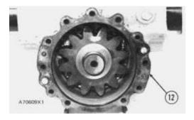
10. Remove shims (12). Put identification on shims for correct installation.
