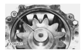
**13.** Put pinion (12) in the housing with the timing mark on the pinion in alignment with timing mark on the rack. See Specifications.
