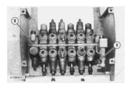
**8.** Remove four bolts and lockwashers (9). Remove control valve (8). Use two persons or a hoist. Weight is 106 lb. (47.7 kg).
