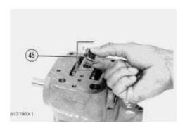
**14.** Install torque control group (45) on the governor housing as shown. Bend the lock to hold the bolts tight.
