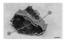
11. Remove shaft (22) and lever (23) from the housing.
