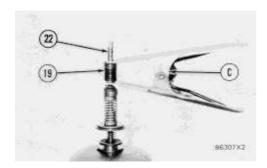
11. Use tool (C) to hold spring (19) in compression, and install ring (22) in the groove in the governor shaft. Remove tool (C).
