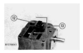
**8.** Remove bolts (12) and torque control (13) from the governor housing.
