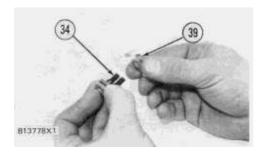
**b.** Install contact (39) on bolts (34) as shown.
