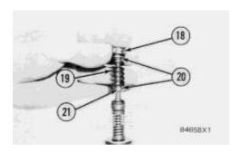
**10.** Install ring (21) in the lower groove in the governor shaft. Install one sleeve (20), spring (19), the other sleeve (20) and bearing (18) on the governor shaft as shown.
