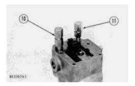
7. Remove high idle adjustment screw (11) and low idle adjustment screw (10) from the governor housing. Remove the high idle adjustment screw first.
