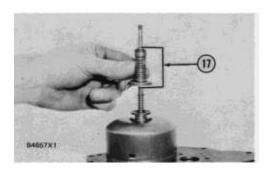
**9.** Install dashpot assembly (17) on the governor shaft as shown.
