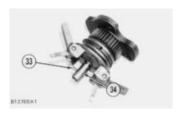
17. Remove the second dowel (33) that holds sleeve (34) in place, and remove the sleeve.
