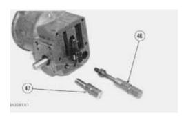
**15.** Install low idle adjustment screw (46) first; then high idle adjustment screw (47) in the governor housing.
