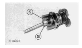
14. Remove ring (27) and the dowel under the ring that holds seat (28) in place.
