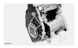
**37.** Remove races (74) and bearing (75) from the camshaft in the fuel injection pump housing.
