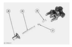
**15.** Remove seat (28), bolt (29) and spring (30) from the weight assembly. Remove washer (31) from spring (30).
