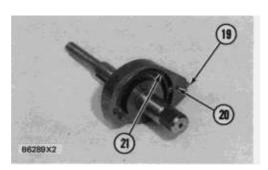
10. Remove pin (20), pin (19) and spring (21) from the shaft assembly.
