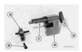
**18.** Install bolt (38) in block (40) as shown. Install spring (37) on bolt (38) as shown. Put collar (34) in position on bolt (38) with the hole in the collar in alignment with the notch in bolt (38), and install bolt (39) to hold the collar in place.
