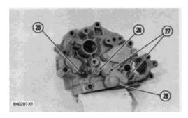
**13.** Remove contact (25) and body (26) for the governor dashpot adjustment screw from the housing. Remove bolts (27), cover (28) and the gasket from the housing.
