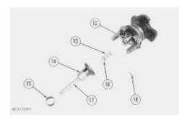
**5.** Install washer (16) in spring (13). Install bolt (17) in seat (14). Put spring (13) and seat (14) in position on guide (12) with the hole in seat (14) in alignment with the hole in guide (12). Install dowel (18) through seat (14) and guide (12). Install ring (15) on the seat to hold the dowel in place.
