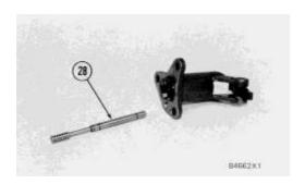
**14.** Install valve (28) in the governor servo as shown.
