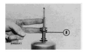
7. Install riser (8) and the spring (overfueling spring) on the governor shaft as shown.
