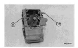
7. Remove low idle adjustment screw (12) and spring (11) from the housing.
