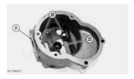
**11.** Remove seal (21) from the governor housing. Use tooling (A) to remove the plug and bearings (20) from the governor housing.
