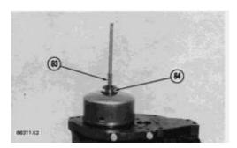
31. Remove spring (overfueling spring) (63) and riser (64) from the governor shaft.
