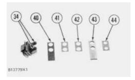
c. Install spring (40), spacer (41), shim (42), bar (43) and insulator (44) on bolts (34) as shown.
