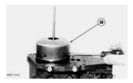
**33.** Use a screwdriver to remove shield (68) as shown.
