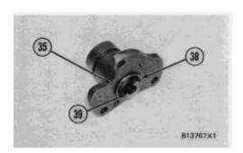
20. Remove sleeve (38) and piston (39) from cylinder (35). Remove the O-ring seal from the sleeve.
