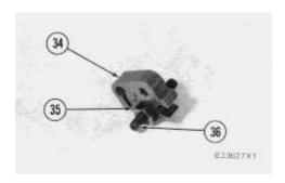
17. Install torque rise adjustment screw (36) in collar (34) as shown, and install locknut (35) on the screw.
