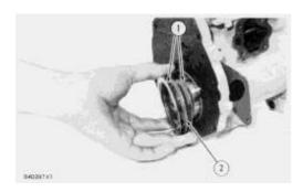
**1.** Install one race (1), bearing (2) and the other race (1) on the camshaft in the fuel injection pump housing.
