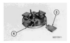
**2.** Put flyweights (3) in position on carrier (4), and install the dowels to hold the flyweights in place. The flyweights must move freely on the dowels and have 0.010 to 0.23 mm (0.0004 to 0.009 in.) end play.
