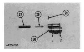
**9.** Put plunger (28) and spring (27) in position in lever assembly (30), and install pin (29) to hold the spring and plunger in place.
