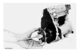
**4.** Put the carrier in position on the camshaft, and install the bolts that hold the carrier in place.
