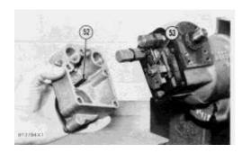
19. Put the gasket and cover in position on the governor housing with dowel (52) in the cover in alignment with notch (53) in the rack stop collar. Install the bolts that hold the cover in place.
