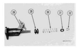
**15.** Install one lockring (32) in the groove near the center of valve (28). Put sleeve (29), spring (broken link spring) (30) and seat (31) in position on valve (28), and install the other lockring (32) to hold them in place.
