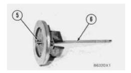
**3.** Install dowel (5) in governor shaft (6), and install the governor shaft in the carrier as shown.
