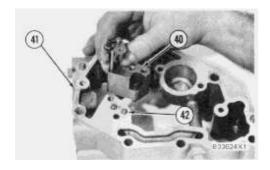
**19.** Put block (40) in position on housing (41) with the holes in the block in alignment with dowels (42). Install the bolts that hold the block in place.
