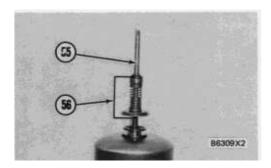
28. Remove ring (55) and dashpot assembly (56) from the governor shaft.
