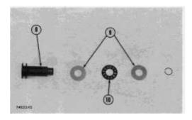
**6.** Install one race (9), bearing (10), the other race (9), and use tool (B) to install the ring on riser (8) as shown.
