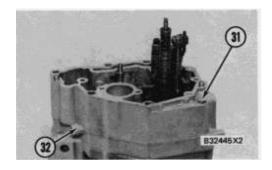
15. Remove two bolts (31), housing (32) and the gasket from the fuel injection pump housing.
