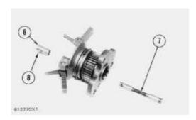
**3.** Install valve (7) through the cylinder, and install sleeve (6) on the valve with the second hole in the sleeve in alignment with the hole in the valve. Install dowel (8) to hold the sleeve on the valve.
