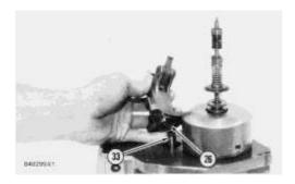
**16.** Put the governor servo in position on the fuel injection pump housing with piston (26) engaged over rack (33), and install the bolts that hold the governor servo in place.
