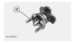
**16.** Remove guide (32), the two races and bearing from the sleeve.
