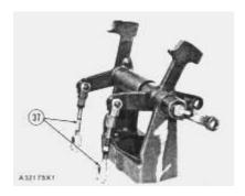
**25.** Remove tilt valve spool and lift valve spool control rods (37).
