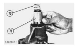
**45.** Remove spring (70) and lift circuit make-up valve (71) from the housing.
