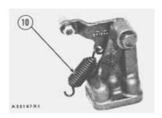
**8.** Remove lift control lever spring (10).
