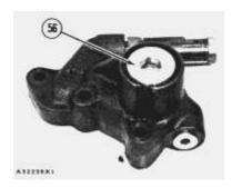
**36.** Remove plug (56) and the seal from the tilt circuit make-up valve.
