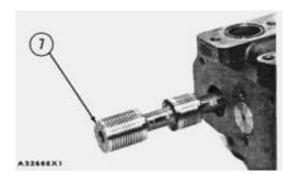
**4.** Install lift cylinder spool (7) in the valve body as shown.
