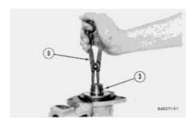
**8.** Use tool (D) to install snap ring (3) in the groove in the camshaft.
