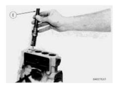
**14.** Use tool (E) to install the fuel injection pump. Installation is made easier by rotation of the cam lobe away from the lifter assembly.
