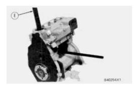
**4.** Install tooling (E) and remove the fuel injection pump.
