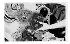
**4.** Install camshaft gear (3) with the "C" mark on the camshaft gear in alignment with the "C" mark on the crankshaft gear. Install the washers and bolts that hold the gear in place.
