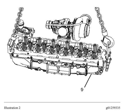
6. Attach a suitable lifting device onto cylinder head (9). The weight of cylinder head (9) is approximately 108 kg (238 lb). Remove cylinder head (9) and the gasket.
