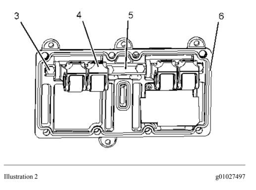
4. Remove bolts (3) and the dowels that hold lifter arms (4) and lifter shaft (5) to each side cover. Remove gasket (6).
