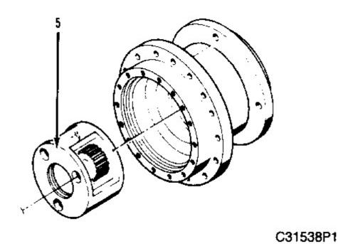
**18.** Install carrier (5) into the torque hub. Make sure the internal spline of the carrier engages the spline of the spindle or output shaft inside the hub.
