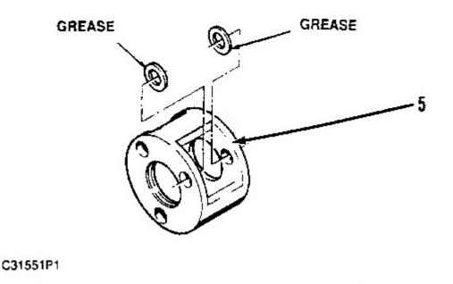
**5.** Apply grease to the tang side of the two thrust washers. Place the thrust washers against bosses in carrier (5). Washer tangs must fit into slots in carrier's outside diameter.
