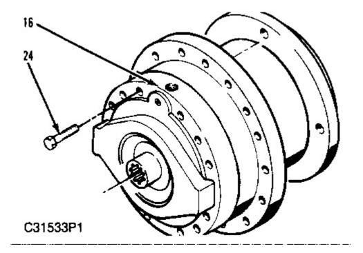
**26.** Install eight standard bolts (24) into the torque hub cover as shown. Tighten the bolts to 31 to  $36 \text{ N} \cdot \text{m}$  (23 to 27 lb ft).
