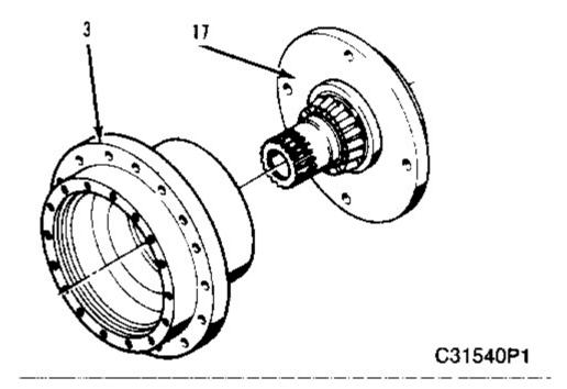
**12.** Press spindle or output shaft (17) out of hub (3).
