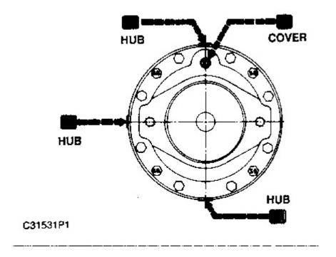
**2.** Remove one or more plugs to drain lubricant from the torque hub. Replace the plug after lubricant has drained.
