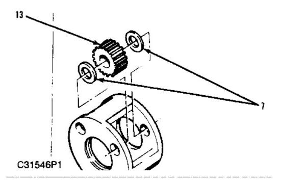
**18.** Remove planet gear (13) and two thrust washers (7) from the carrier.
