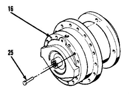
**25.** Install four shoulder bolts (25) into the torque hub cover as shown. Tighten the bolts to 31 to  $36 \text{ N} \cdot \text{m}$  (23 to 27 lb ft).
