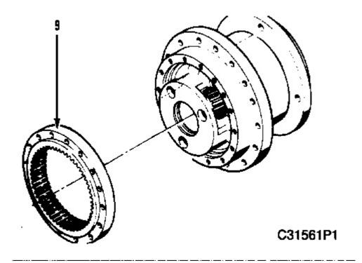
**19.** Slide ring gear (9), with the shoulder side toward the hub, into mesh with the planet gears. Be sure to align the scribe marks made during disassembly.
