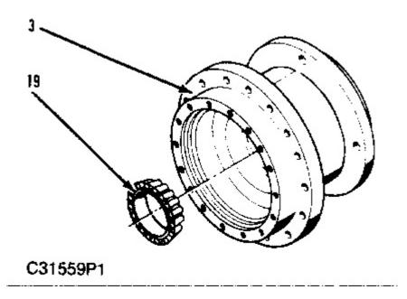
**14.** Press outer bearing cone (19) on the spindle or output shaft inside hub (3). Rotate the hub while pressing the bearing. Stop pressing when the hub starts to resist rolling.
