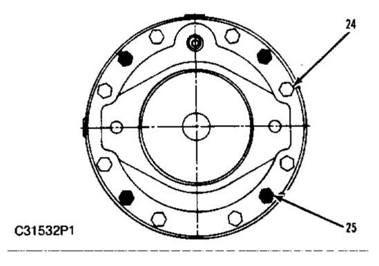
**NOTE:** The cover is secured to the torque hub with eight standard bolts (24) and four shoulder bolts (25). These bolts are positioned in the cover as shown above.
