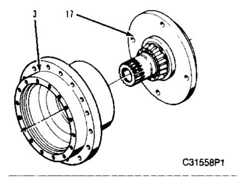
**13.** Carefully raise hub (3) and set in place on spindle or output shaft (17). Use care to prevent damaging the seal, if installed.
