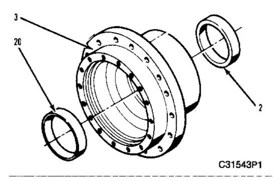
15. Press two bearing cups (2) and (20) out of hub (3).
