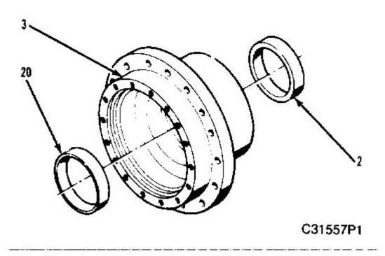
12. Press inner bearing cup (2) and outer bearing cup (20) in place inside hub (3).
