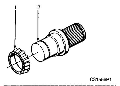
11. If the torque hub uses an output shaft (17), as shown above, press inner bearing cone (1) onto the output shaft. Seal (18) will be installed in a later step.
