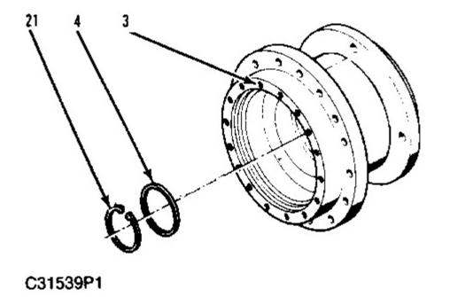
**15.** Install spacer (4) so that it rests on top of the outer bearing cone.
