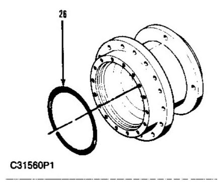
**17.** Apply a light coat of grease to one new O-ring (26). Install the O-ring into the counter-bore of the hub.
