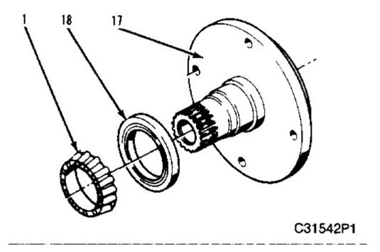
**14.** Pull inner bearing cone (1) and seal (18) off spindle or output shaft (17). Discard seal (18). This must be replaced with a new part during assembly.
