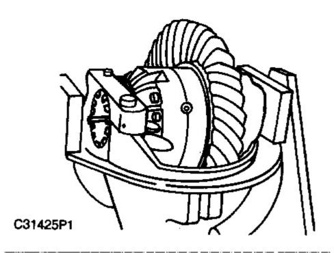
**6.** Turn the differential and carrier as shown. Remove the bolts and washers securing the lock plates at each side of the differential. Remove the lock plates.
