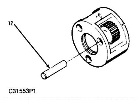
7. Install one planet shaft (12) through the carrier and planet gear. Line up the roll pin hole in the planet shaft with the carrier roll pin hole.
