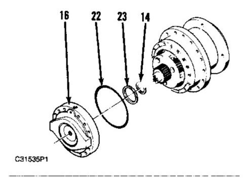
**5.** Remove cover (16), one O-ring (22), and two thrust washers (23) and (14) off the torque hub. Discard O-ring (22). This must be replaced with a new part during assembly.
