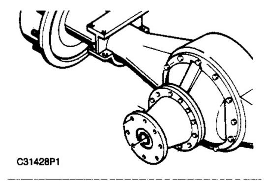
**3.** Remove the nuts, bolts, and washers securing the adapter housing to the axle. Remove the adapter housing.
