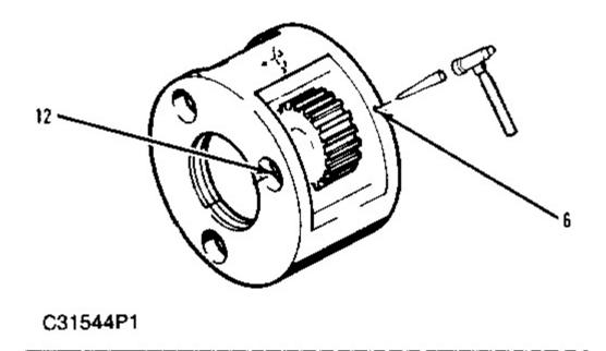
**16.** Drive roll pin (6) out of one of the planet shafts (12).
