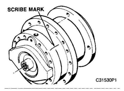
**1.** Make matching scribe marks on the cover, ring gear, and hub. This will help ensure that these parts are reassembled in their original positions.
