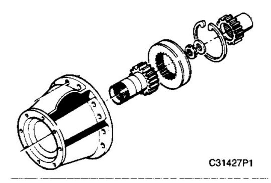
4. Remove the snap ring, gear coupler, and adapter gear from inside the adapter housing.
