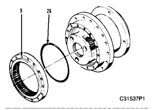
**7.** Remove ring gear (9) and remaining O-ring (26). Discard O-ring (23). This must be replaced with a new part during assembly.
