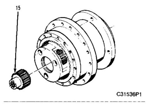
**20.** Slide input gear (15) into mesh with the planet gears inside the carrier until it rests against the shoulder.
