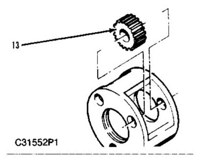
**6.** When the thrust washers are in place, slide planet gear (13) between them. Line up the planet gear bore with the hole in the carrier.
