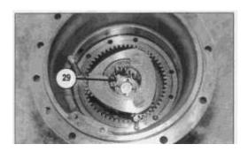
**24.** Remove lock (29) from the axle retainer bolt.
