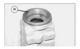
**33.** Remove bearing cup (45) from the housing.
