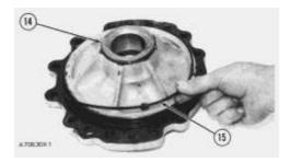
**15.** If the bearing was removed, put a support under the cover and install bearing (14) with a press.
