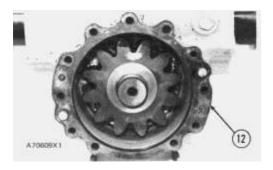
**10.** Remove shims (12). Put identification on shims for correct installation.
