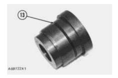
12. Remove O-ring seal and back-up seal (13) from the head.
