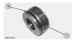
10. Remove seal assembly (10) and wear ring (11) from the piston.
