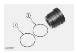
**8.** Install back-up ring (5) and O-ring seal (6) on the head.
