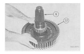
**5.** Install gear (17) on sprocket shaft (6). Install the bolts and nuts that hold the gear and sprocket together. Tighten the nuts to a torque of  $80 \pm 7 \text{ N} \cdot \text{m}$  ( $60 \pm 5 \text{ lb ft}$ ). Turn the nuts an additional  $120^{\circ} \pm 5^{\circ}$ . Minimum torque must be 307 N·m (230 lb ft).
