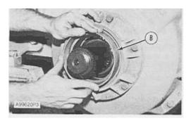
**NOTE:** The rubber seals and all surfaces that make contact with the seals must be clean and dry with no damage to the surface. After installation of the seals, put oil on the contact surfaces of the Duo-Cone seals.
