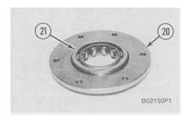
**NOTE:** Do not remove race and roller assembly (21) unless a replacement is needed. The bearing can be damaged when removed.
