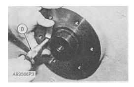
**5.** Install tooling (D) to check the distance from the shoulder of the sprocket shaft to the face of the sprocket hub. The distance must be  $3.00 \pm 0.8$  mm (.118  $\pm$  .03 in).
