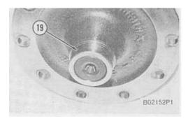
15. If a replacement is needed, remove bearing race (19) from the sprocket shaft.
