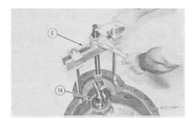
**NOTE:** Do not remove race and roller assembly (14) unless a replacement is needed. The bearing can be damaged when removed.
