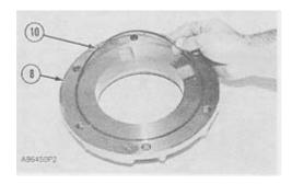
**12.** Inspect O-ring seal (10) for damage and make a replacement if needed. Install O-ring seal (10) on retainer (8).
