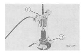
**14.** Remove bearing cone (18) from the sprocket shaft with tooling (F).
