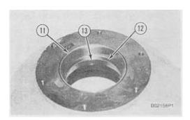
**10.** If a replacement is needed, remove bearing cup (11), spacer (12) and bearing cup (13) from the cover.
