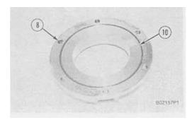
**9.** Remove O-ring seal (10) from retainer (8).
