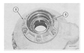
**8.** Remove retainer (8) and bearing cone (9) from the cover.
