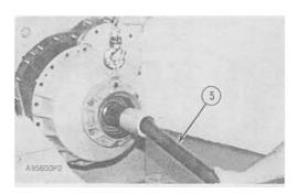
**15.** Fasten a hoist to tooling (J). Put 138-8436 Liquid Gasket Material on the cover and the steering clutch case that makes contact with each other. Install bar (5) in the 5P6514 Adapter to put the sprocket shaft, gear and cover in balance. Install the unit on the steering clutch case. Install the nuts and bolts that hold the cover to the steering clutch case.
