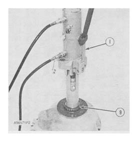
**11.** Use tooling (I) as shown and install bearing cone (9) on the sprocket shaft with a force of 178 to 240 kN (20 to 27 ton). Turn the cover to put the bearing cones on their seats in the bearing cups.
