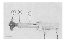
**4.** Install bearing cone (18) on sprocket shaft (6) with tooling (I). Use a force of 98 to 240 kN (11 to 27 ton).
