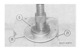
1. Install race and roller assembly (21) in bearing cage (20) with tooling (G) and a press.
