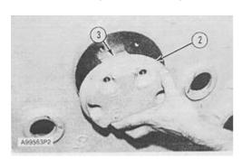
**8.** Put 138-8436 Liquid Gasket Material between locknut (2) and the sprocket hub face. Install locknut (2). If the bolt holes do not make an alignment with the holes in the sprocket hub, turn nut (3) clockwise only enough to install locknut (2).
