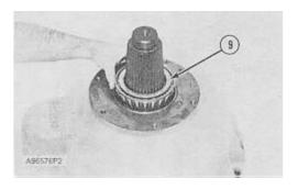
**10.** Put bearing cone (9) in position on the sprocket shaft.
