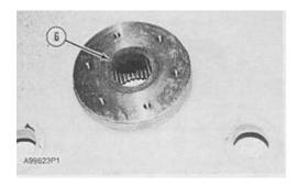
**6.** Remove gasket (6) from the sprocket hub.
