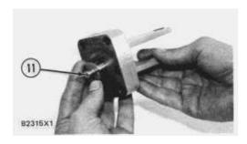
7. Pull stem (11) in until it can be turned. Turn the stem 90° and push it out until it hits the pin.
