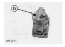
10. Remove the bolt and cover (15) from the valve.
