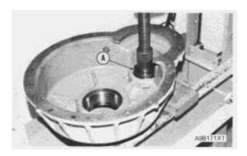
7. If the race and roller assembly was removed, install the race and roller in the cover with tooling (A) and a press.
