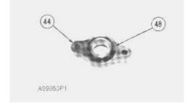
23. Remove O-ring seal (48) from spacer (44).
