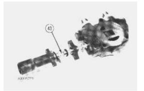
**21.** Remove lift control valve spool (43) from the lift control valve body.
