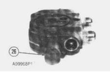
**11.** Remove cap (26) from the other end of the tilt control valve body.
