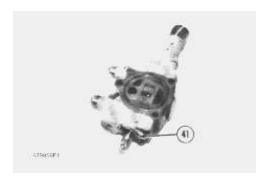
**19.** Remove plate (41) and the wiper seal behind the plate. Remove O-ring behind the wiper seal.
