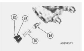
**5.** Install O-ring seal (63) on plug (62). Install check valve (64), spring (65), and plug (62) in the lift control valve body.
