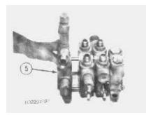
**3.** Remove inlet oil manifold (5) from the rods.
