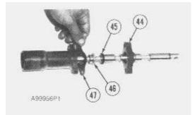
**22.** Remove spacer (44), O-ring seal (45), wiper seal (46) and plate (47) from the lift control valve spool.
