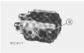
**34.** Remove O-ring seal (72) from the lift control valve body.
