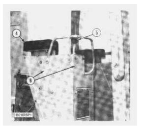
**3.** Remove knob (5) from the control lever. Remove arm cushion and bracket (4). Remove cover assemblies (6) and the guard as a unit.
