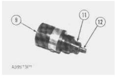
c. Remove plunger (12) and orifice (11) from valve body (9).
