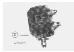
**12.** Remove tilt control valve spool (27) from the tilt control valve body.
