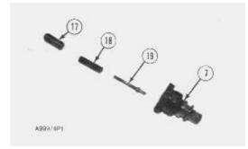
f. Remove adjustment screw (17), spring (18) and plunger (19) from valve body (7).
