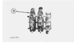
6. Remove tilt control valve (20) from the rods.
