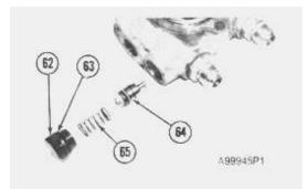
**32.** Remove plug (62), spring (65) and check valve (64) from the lift control valve body. Remove Oring seal (63).
