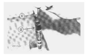
26. Put the flat end of the lift control valve spool in a vise.
