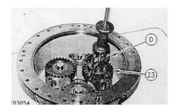
17. Using Tooling (D), remove gear assembly (23).
