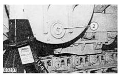
1. Remove plugs (1) and (2) and drain the fluid from the final drive. The capacity of the final drive is 20.5 L (5.5 gal U.S.). Install plugs (1) and (2) in the final drive.
