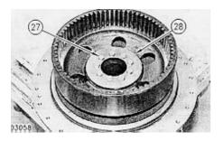
23. Remove nine bolts (27) and retainer (28) from the final drive assembly.
