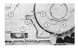
**2.** Remove three bolts (3), washers and guard (4). Remove three bolts (5), washers and guard (6). Remove four bolts (7), washers and guard (8).
