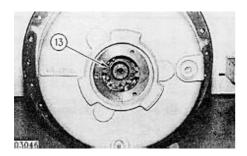
**9.** Remove shaft (13) by pushing the shaft from the opposite side.
