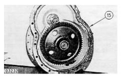
**9.** Clean surfaces (14) and (15). Apply a 3-4 mm wide bead of **6V-6640 sealant**to the final drive assembly as shown.
