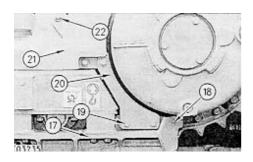
**12.** Install guard (18), four bolts (17) and washers. Install cover (21), three bolts (22) and washers. Install cover (20), three bolts (19) and washers.
