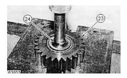
18. Using a suitable press, remove shaft assembly (24) from gear assembly (23).
