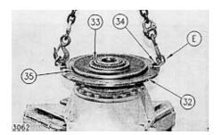
27. Remove bearing (33) and O-ring seal (35). Install Tooling (E) and two 1/2 X 1-1/2bolts (34), and washers. Using a suitable lifting device, remove hub assembly (32). The weight of the hub assembly is 64 Kg (140 lb). Remove Tooling (E).
