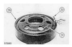
**25.** Remove ring (30) and hub (31) from gear (30).
