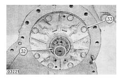
**16.** Remove gear assembly (32), eight bolts (33) and washers.
