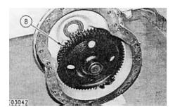
**5.** Remove gear assembly (8) from the final drive assembly.
