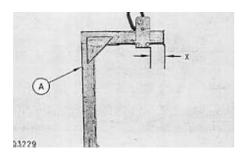
7. Adjust the bracket on Tooling (A) until dimension (X) is 225 mm (9 in).
