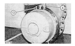
**8.** Attach Tooling (A) to a hoist and to the final drive assembly using two 1/21/4 - **20 X 2**bolts (13) and washers.
