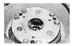
15. Remove six bolts (20) and washers from the carrier assembly.
