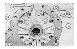
**17.** Install two **M12 X 40 mm**pusher bolts (35) and remove cage assembly (36). If necessary remove and replace two dowels (34) and two dowels (37).
