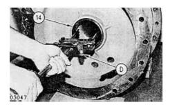
**10.** Using Tooling (D), remove race (14).
