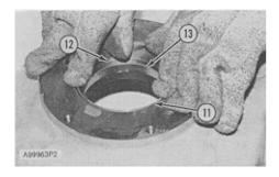
**6.** Lower the temperature of bearing cups (13) and (11). Install bearing cup (13), spacer (12) and bearing cup (11) in the cover.
