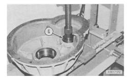
7. If the race and roller assembly was removed, install the race and roller in the cover with tooling (G) and a press.
