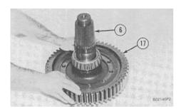
5. Install gear (17) on sprocket shaft (6). Install the bolts and nuts that hold the gear and sprocket shaft together. Tighten the nuts to a torque of  $80 \pm 7 \text{ N} \cdot \text{m}$  ( $60 \pm 5 \text{ lb ft}$ ). Turn the nuts an additional  $120^{\circ} \pm 5^{\circ}$ . Minimum torque must be  $307 \text{ N} \cdot \text{m}$  (230 lb ft)
