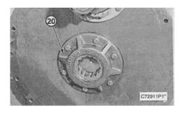
**16.** Remove bearing cage (20) from the steering clutch case.
