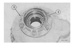
**8.** Remove retainer (8) and bearing cone (9) from the cover.
