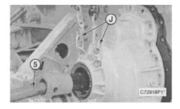
15. Fasten a hoist to tooling (J). Put 6V6440 Liquid Gasket Material on the cover and the steering clutch case that makes contact with each other. Install bar (5) in the 5P6514 Adapter to put the sprocket shaft, gear and cover in balance. Install the unit on the steering clutch case. Apply 9S3263 Thread-Lock to the threads of bolts (1) (not shown) that hold the cover to the steering clutch case. Tighten the bolts to a torque of  $135 \pm 150 \text{ N*m}$  ( $100 \pm 11 \text{ lb ft}$ ).
