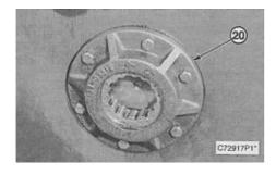
**2.** Install bearing cage (20) on the steering clutch case.
