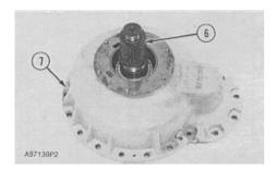
**8.** Put sprocket shaft (6) and gear on wooden block. Put cover (7) in position on the sprocket shaft and gear.
