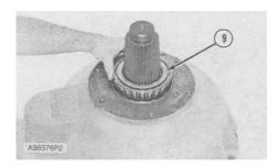
**10.** Put bearing cone (9) in position on the sprocket shaft.
