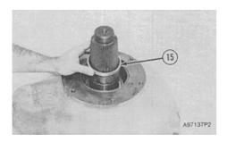
**9.** Install spacer (15) on the sprocket shaft.
