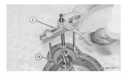
**NOTE:** Do not remove race and roller assembly (14) unless a replacement is needed. The bearing can be damaged when removed.
