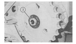
7. Install nut (3) that holds the sprocket hub on the sprocket shaft. Tighten the nut to a torque of  $334 \pm 33 \text{ N} \cdot \text{m} (243 \pm 24 \text{ lb ft})$
