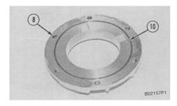
**9.** Remove O-ring seal (10) from retainer (8).
