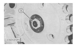
**3.** Remove nut (3) from the sprocket shaft.
