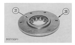
**NOTE:** Do not remove race and roller assembly (21) unless a replacement is needed. The bearing can be damaged when removed.
