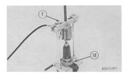
**14.** Remove bearing cone (18) from the sprocket shaft with tooling (F).
