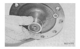
**3.** If bearing race (19) was removed, heat bearing race (19) to a maximum temperature of **135° C** (275° F). Install bearing race (19) on the sprocket shaft. If necessary, use tooling (H) to install the bearing race.
