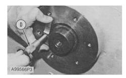
5. Use tooling (D) to check the distance from the shoulder of the sprocket shaft to the face of the sprocket hub. The distance must be  $3.00 \pm 0.8 \text{ mm}$  (.118  $\pm .03 \text{ in}$ ).
