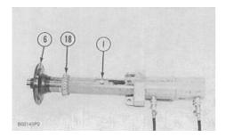
**4.** Install bearing cone (18) on sprocket shaft (6) with tooling (I). Use a force of **98 to 240 kN (11 to 27 ton).**
