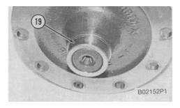
15. If a replacement is needed, remove bearing race (19) from the sprocket shaft.
