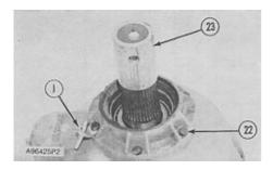
**14.** Install bolts (22) and tooling (J). Install **5P6514 Adapter** (23) [part of tooling (I)] on the end of the sprocket shaft.
