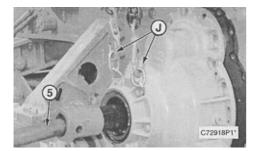
15. Fasten a hoist to tooling (J). Put 6V6440 Liquid Gasket Material on the cover and the steering clutch case that makes contact with each other. Install bar (5) in the 5P6514 Adapter to put the sprocket shaft, gear and cover in balance. Install the unit on the steering clutch case. Apply 9S3263 Thread-Lock to the threads of bolts (1) (not shown) that hold the cover to the steering clutch case. Tighten the bolts to a torque of  $135 \pm 150$  N\*m ( $100 \pm 11$  lb ft).
