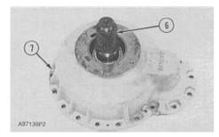
**8.** Put sprocket shaft (6) and gear on wooden block. Put cover (7) in position on the sprocket shaft and gear.
