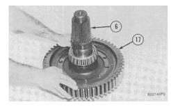
5. Install gear (17) on sprocket shaft (6). Install the bolts and nuts that hold the gear and sprocket shaft together. Tighten the nuts to a torque of  $80 \pm 7$  N·m ( $60 \pm 5$  lb ft). Turn the nuts an additional  $120^{\circ} \pm 5^{\circ}$ . Minimum torque must be 307 N·m (230 lb ft)
