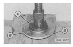
**1.** Install race and roller assembly (21) in bearing cage (20) with tooling (G) and a press.
