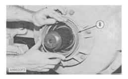
**NOTE:** The rubber seals and all surfaces that make contact with the seals must be clean and dry with no damage to the surface. After installation of the seals, put oil on the contact surfaces of the Duo-Cone seals.
