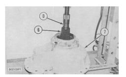
6. Remove sprocket shaft (6) and gear from cover (7) with tooling (D) and a press.
