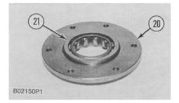
**NOTE:** Do not remove race and roller assembly (21) unless a replacement is needed. The bearing can be damaged when removed.
