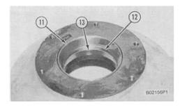
10. If a replacement is needed, remove bearing cup (11), spacer (12) and bearing cup (13) from the cover.
