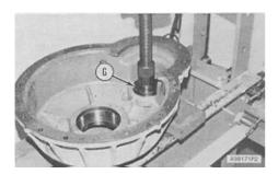
7. If the race and roller assembly was removed, install the race and roller in the cover with tooling (G) and a press.
