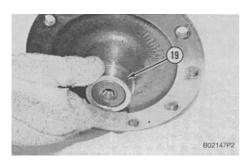
**3.** If bearing race (19) was removed, heat bearing race (19) to a maximum temperature of **135° C** (**275° F).** Install bearing race (19) on the sprocket shaft. If necessary, use tooling (H) to install the bearing race.
