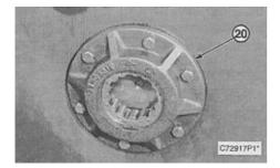
**2.** Install bearing cage (20) on the steering clutch case.
