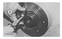
**5.** Use tooling (D) to check the distance from the shoulder of the sprocket shaft to the face of the sprocket hub. The distance must be  $3.00 \pm 0.8 \text{ mm}$  (.118 ± .03 in).
