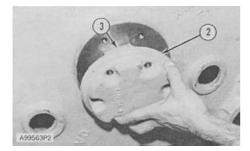
**8.** Put **7M7260 Liquid Gasket Material** between the locknut (2) and the sprocket hub face. Install locknut (2). If the bolt holes do not make an alignment with the holes in the sprocket hub, turn nut (3) clockwise only enough to install locknut (2).
