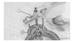
**NOTE:** Do not remove race and roller assembly (14) unless a replacement is needed. The bearing can be damaged when removed.
