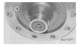
15. If a replacement is needed, remove bearing race (19) from the sprocket shaft.
