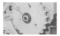
7. Install nut (3) that holds the sprocket hub on the sprocket shaft. Tighten the nut to a torque of  $334 \pm 33$  N·m (243 ± 24 lb ft)
