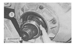
**16.** Put oil on the threads and friction material of locknut (1). If oil is not used, the friction material will be destroyed when it is put on the threads of the sprocket shaft.
