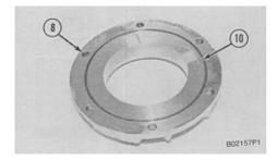
9. Remove O-ring seal (10) from retainer (8).
