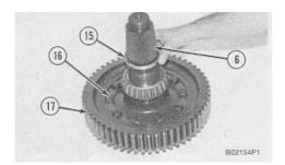
12. Remove spacer (15) from the sprocket shaft (6).
