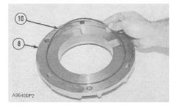
**12.** Inspect O-ring seal (10) for damage and make a replacement if needed. Install O-ring seal (10) on retainer (8).
