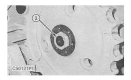
**3.** Remove nut (3) from the sprocket shaft.
