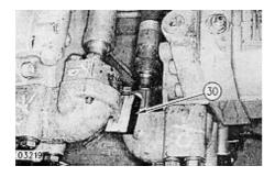
14. Install wood block (30) between the two drive motors as shown.
