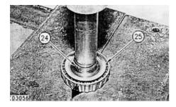
19. Using a suitable press, removes shaft (24) from bearing (25).
