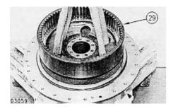
**24.** Using a suitable lifting device, remove gear assembly (29). The weight of the gear assembly is **27 Kg (60 lb).**
