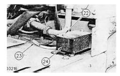
**11.** Remove two bolts (22) and washers. Disconnect wire connector (23) and remove back up alarm assembly (24).
