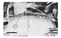
13. Cut strap (28) and remove eight bolts (27), washers and plate (29).
