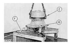
**12.** Using a suitable lifting device and Tooling (E), position the final drive assembly on Tooling (F). Install four **M16 X 60 mm**bolts (16), washers and nuts. Remove Tooling (E).
