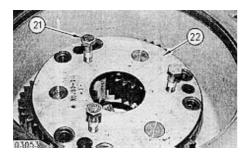
16. Install three M16 X 60 mmpusher bolts (21) and remove plate (22).
