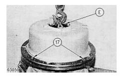
**13.** Install Tooling (E) as shown using three **M10 X 35 mm**bolts and washers. Attach a suitable lifting device and remove four bolts (17).
