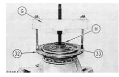
26. Install Tooling (G) and (H) as shown. Pull hub assembly (32) and bearing (33) from its seat.
