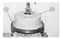
14. Install two M12 X 175 mmpusher bolts (18) and remove carrier assembly (19). The weight of the carrier assembly is 75 Kg (165 lb).
