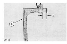
7. Adjust the bracket on Tooling (A) until dimension (X) is 225 mm (9 in).
