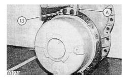
**8.** Attach Tooling (A) to a hoist and to the final drive assembly using two 1/21/4 - **20 X 2**bolts (13) and washers.
