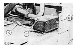
6. Install back up alarm assembly (12), two bolts (11) and washers. Connect wire connector (10).
