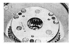
15. Remove six bolts (20) and washers from the carrier assembly.
