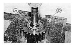
18. Using a suitable press, remove shaft assembly (24) from gear assembly (23).
