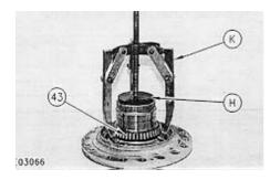
**34.** Using Tooling (H) and (K), remove bearing cone (34).
