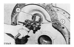
11. Using Tooling (D), remove bearing (15).
