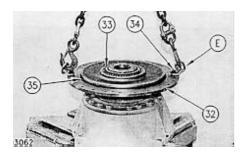
**27.** Remove bearing (33) and O-ring seal (35). Install Tooling (E) and two 1/2 X 1-1/2bolts (34), and washers. Using a suitable lifting device, remove hub assembly (32). The weight of the hub assembly is 64 Kg (140 lb). Remove Tooling (E).
