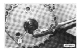
7. Use tool (F) to install the nut that holds the sprocket on the sprocket shaft. Tighten the nut to a torque of  $334 \pm 33 \text{ N} \cdot \text{m}$  ( $243 \pm 24 \text{ lb.ft.}$ ).
