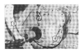
**5.** Install two 3/8 " - 16 NC forcing screws (4). Tighten the forcing screws evenly and remove the sprocket shaft, gear and cover as a unit. Use bar (5) inside of tool (B) to keep the unit in balance when it is removed. The weight is 108 kg (240 lb.).
