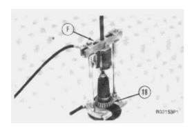
**14.** Remove bearing cone (18) from the sprocket shaft with tooling (F).
