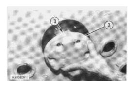
**8.** Put 7M7260 Liquid Gasket Material between locknut (2) and the sprocket face. Install locknut (2). If the bolt holes do not make an alignment with the holes in the sprocket, turn nut (3) clockwise only enough to install locknut (2).
