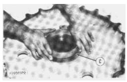
**2.** Install the outer half of the Duo-Cone seal in the sprocket with tool (C).
