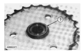
**7.** Remove outer half of Duo-Cone seal (7) from the sprocket.
