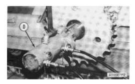
**4.** Install tooling (D) and fasten a hoist. Use tooling (D) to install the sprocket on the sprocket shaft with a force of 311 to 355 kN (35 to 40 ton).
