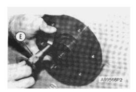
**5.** Use tooling (E) to check the distance from the shoulder of the sprocket shaft to the face of the sprocket. The distance must be  $3.00 \pm 0.8$  mm (.118  $\pm$  .03 in.).
