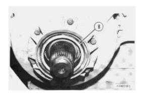
**8.** Remove inner half of Duo-Cone seal (8) from the retainer.
