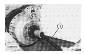
**15.** Fasten a hoist to tooling (J). Put 7M7260 Liquid Gasket Material on the cover and the steering clutch case that makes contact with each other. Install bar (5) in the 5P6514 Adapter to put the sprocket shaft, gear and cover in balance. Install the unit on the steering clutch case. Install the nuts and bolts that hold the cover to the steering clutch case.
