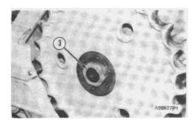
**3.** Use tool (B) to remove nut (3) from the sprocket shaft.
