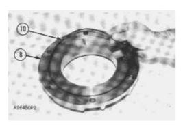
**12.** Inspect O-ring seal (10) for damage and make a replacement if needed. Install O-ring seal (10) on retainer (8).
