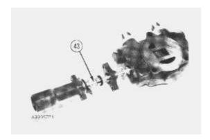
**21.** Remove lift control valve spool (43) from the lift control valve body.
