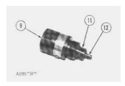
c. Remove plunger (12) and orifice (11) from valve body (9).
