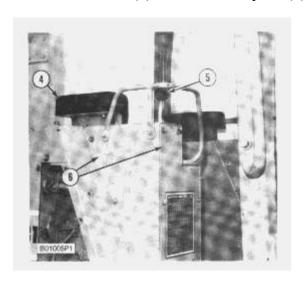
**3.** Remove knob (5) from the control lever. Remove arm cushion and bracket (4). Remove cover assemblies (6) and the guard as a unit.
