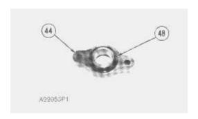
23. Remove O-ring seal (48) from spacer (44).
