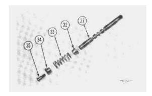
15. Remove screw (35), seat (34), spring (33) and seat (32) from tilt control valve spool (27).
