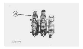
**6.** Remove tilt control valve (20) from the rods.
