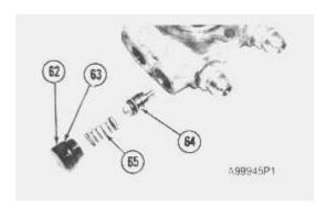
**32.** Remove plug (62), spring (65) and check valve (64) from the lift control valve body. Remove O-ring seal (63).
