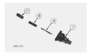
**f.** Remove adjustment screw (17), spring (18) and plunger (19) from valve body (7).
