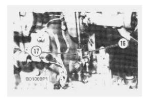
11. Connect control linkages (16) and (17) to the hydraulic control valves.
