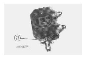
**12.** Remove tilt control valve spool (27) from the tilt control valve body.
