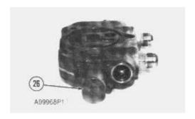
11. Remove cap (26) from the other end of the tilt control valve body.
