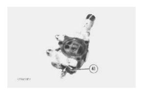
19. Remove plate (41) and the wiper seal behind the plate. Remove O-ring behind the wiper seal.
