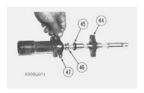
**22.** Remove spacer (44), O-ring seal (45), wiper seal (46) and plate (47) from the lift control valve spool.
