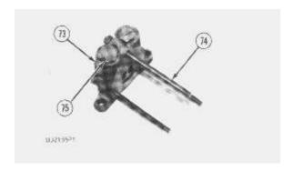
**35.** Remove rods (74) from the outlet manifold (73). Remove plugs (75) and O-ring seals from the outlet manifold.
