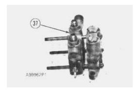
17. Remove lift control valve (37) from the rods.
