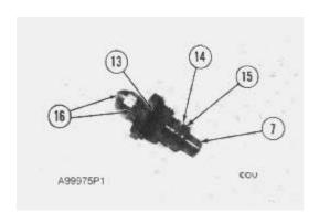
**d.** Remove O-ring seal (15), ring (14) and O-ring seal (13) from valve body (7).
