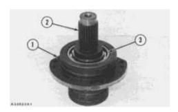
**3.** Install shaft (2) and bearing (3) in cage (1).
