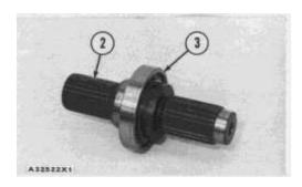
**2.** Heat bearing (3) in oil to a maximum temperature of  $275^{\circ}$  F ( $135^{\circ}$  C). Install bearing (3) on shaft (2).
