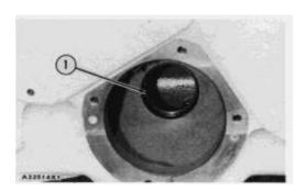
1. Inspect ring (1) in case. Make a replacement if necessary.
