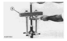
**4.** Remove the bearing from the shaft with tooling (B).
