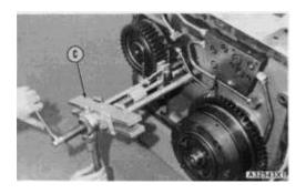
**9.** Remove the bearing cup from the case assembly with tooling (C).
