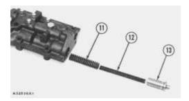
**10.** Remove the cover and remove piston (13), spring (12) and spring (11).
