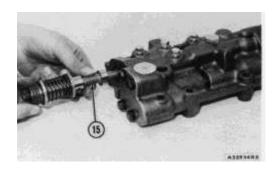
11. Install valve spool (15) and the cover on the control valve body. Tighten bolts to  $22 \pm 3$  lb. ft.  $(30 \pm 4 \ N \cdot m)$ .
