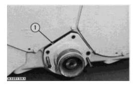
**1.** Remove the bolts from input shaft cage (1). Remove input gear assembly with two 3/8"-16 NC forcing screws.
