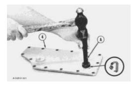
**5.** Put 7M7260 Liquid Gasket material in bore of cover assembly (4). Use tooling (A) and install the seal in cover assembly (4) with lip of seal toward inside.
