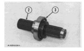
**2.** Heat bearing (3) in oil to a maximum temperature of  $275^{\circ}$  F (135° C). Install bearing (3) on shaft (2).
