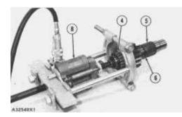
**5.** Remove the carrier and bearing (4) from gear (5) with tooling (B) and remove the seal from the carrier.
