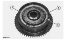
**7.** Remove ring (8), hub (7), thick plate (9), the five disc assemblies, the four plates and the thick plate.
