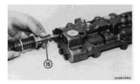
**11.** Install valve spool (15) and the cover on the control valve body. Tighten bolts to  $22 \pm 3$  lb. ft. ( $30 \pm 4 \text{ N} \cdot \text{m}$ ).
