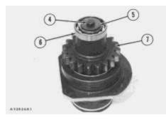
**4.** Install gear (7) on shaft (2).
