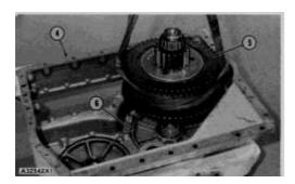
**6.** Use two 3/8"-16 NC forcing screws and remove cage (6) and the shims. Keep the shims together for installation.
