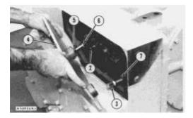
**7.** Install new O-ring seals on sleeve (6). Install sleeve (6) in cover (4). Install the clip on sleeve (6) and tighten bolt (5).
