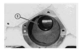
**1.** Inspect ring (1) in case. Make a replacement if necessary.
