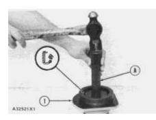
**1.** Use tooling (A) and install the lip-type seal with lip of the seal toward the inside when cage (1) is installed on the winch.
