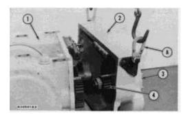
1. Clean the gasket material from the surfaces of the case assembly (1) and case (2).
