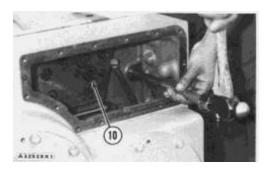
**9.** Fill the bearing in the case assembly with grease and use a .75 in. (19.05 mm) diameter shaft to force the bearing from the case assembly.
