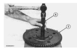
**3.** There is a counterbore in gear (3). Remove the bearing from the counterbore side of gear with tooling (A).
