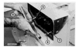
**8.** Install washer (7) on shaft (8). Install a new gasket and install cover (6) on the case. Make sure sleeve (5) fits in control valve before the bolts are tightened.
