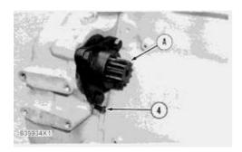
**3.** Install tooling (A) in the flywheel housing.
