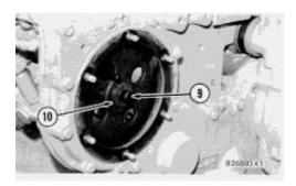
**10.** Loosen bolt (9) that holds the fuel injection pump gear to the sleeve approximately 3.2 mm (.125 in.).
