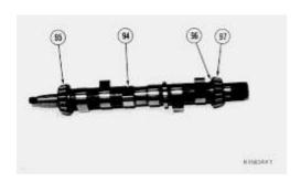
**60.** Remove bearing cones (95) and (97) from fuel injection pump camshaft (94) with tool (J) and a press. Remove shims (96) from behind bearing cone (97).
