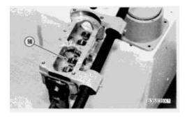
**62.** Remove lifters (98) from the fuel injection pump housing.
