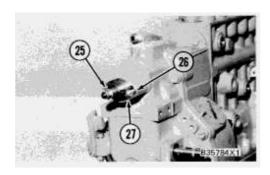
17. Remove studs (25) and (26). Remove rack setting group (27) and the gasket.
