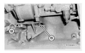
17. Remove bolts (19) that hold the fuel injection pump spacer to bracket (18).
