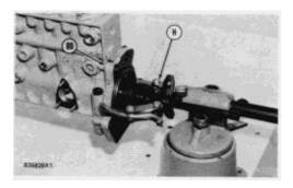
**56.** Use tooling (H) and removed adapter (89).
