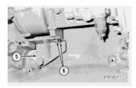
**4.** Install the three nuts that hold the fuel injection pump housing and governor to the timing plate. Install bolts (6) that hold the fuel injection pump spacer to bracket (5).
