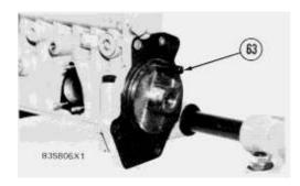
**38.** Turn the fuel injection pump camshaft until the hole in the sleeve is in alignment with the hole in the adapter. Install timing pin (63) so the fuel injection pump camshaft will not turn.
