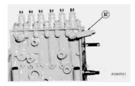
**48.** Remove fuel bypass valve (82) from the fuel injection pump housing.
