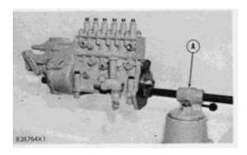
1. Install the fuel injection pump and governor on tooling (A) as shown.
