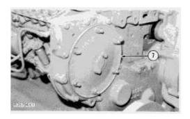
**8.** Remove cover (7) from the front of the timing gear cover.
