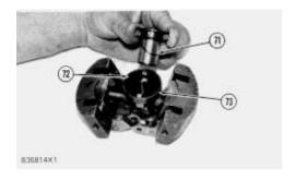
**42.** Remove puller (71) from ring (73). Remove dampers (72) from ring (73). Remove ring (73) from the flyweights.
