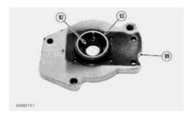
**58.** Remove lip type seal (92) and bearing cup (93) from adapter (89).
