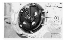
2. Make sure that the centerline of one of the holes in fuel injection pump gear (2) is 30° to the left of the vertical centerline of the fuel injection pump gear. This will permit the timing pin [tool (A)] to go through the hole in the fuel injection pump gear when the fuel injection pump and governor is installed.
