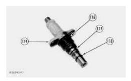
**73.** Remove O-ring seals (116), (117) and (118) from barrel assembly (114).
