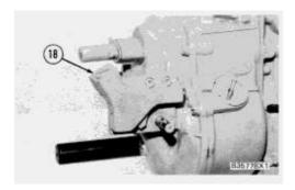
**14.** Remove detent mechanism (18) from the governor cover.
