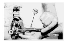
**33.** Move fulcrum lever (55) 90° from the governor housing as shown and remove fulcrum lever (55) and fork (56) from the shaft.
