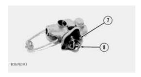
**6.** Remove ring (7) that holds the lifter in place. Remove lifter (8).
