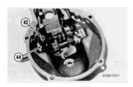
**26.** Remove bolt (43) that holds plate (44) to the governor cover. Remove the shims under the plate.
