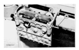
**59.** Pull fuel injection pump camshaft (94) forward just enough to remove center bearing (87). Remove center bearing (87). Remove fuel injection pump camshaft (94).
