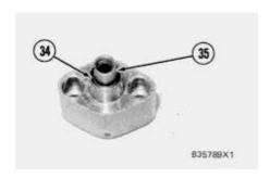
**21.** Remove ring (34) that holds bushing (35) in place. Remove bushing (35) and spring (36) from the adapter.
