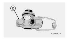
11. Remove plug (15), gasket, spring and valve from the housing.
