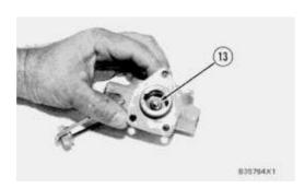
**9.** Push on rod (13) to remove rod (13) and the piston from the other side.
