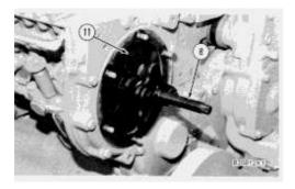
**11.** Install tooling (B) and loosen fuel injection pump gear (11) from the sleeve. Remove tooling (B). Remove bolt (9) and washer (10).
