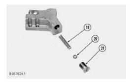
15. Remove screw (21), shim (20) and spring (19) from the detent mechanism.
