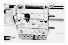
**49.** Turn the fuel injection pump housing over as shown. Remove cover (83) and gasket from the bottom of the fuel injection pump housing.
