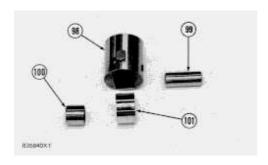
**63.** Remove pins (99) that hold rollers (101) and bushings (100) in the lifters. Remove rollers (101) and bushings (100) from lifters (98).
