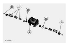
**41.** Use tool (D) and remove nut (66) from each side of the flyweight. Remove seat (70), spring (67), shims (69) and seat (68) from each side of flyweights (65).
