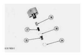
22. Remove ring (38) and remove sleeve (37) from bushing (35).
