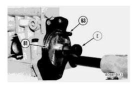
**47.** Use tool (E) and remove sleeve (81). Remove timing pin (63).
