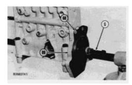
55. Remove bolts (88) that hold adapter (89) to the fuel injection pump housing.
