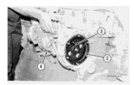
**3.** Install the O-ring seal on the face of the fuel injection pump housing. Put fuel injection pump housing and governor (4) in position on the engine and against the timing gear plate. Make sure timing pin (3) [tool (A)] goes through the hole in the fuel injection pump gear as shown.
