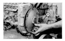
**9.** Put the gasket in place and install cover (9) on the front of the timing gear cover.
