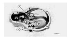
**31.** Remove bearing (52) and seal (53) from each side of the governor cover.
