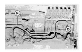
**14.** Remove oil supply line (15) and oil drain line (14).
