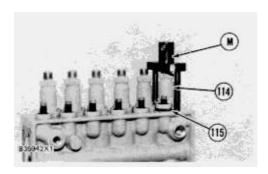
72. Use tool (M) and remove barrel assemblies (114). Remove shims (115).
