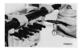
**52.** Turn the fuel injection pump camshaft until the lifter is as far down in the bore as possible. Install tooling (F) with the flat side toward the lifter. Tooling (F) will hold the lifter down when the fuel injection pump camshaft is removed. Do the other lifters the same way.
