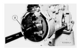
**39.** Use tooling (B) and remove nut (64) that holds the flyweights on the fuel injection pump camshaft. Remove the shim behind the nut.
