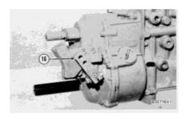
12. Remove lever (16) and the key from the shaft.
