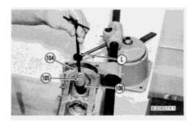
**65.** Use tool (L) and remove springs (104), control sleeves (105) and upper spring seats (106) from the fuel injection pump housing.
