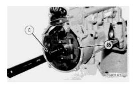
**40.** Use tooling (C) and remove flyweights (65) from the fuel injection pump camshaft.
