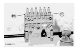
**71.** Remove barrel housing flange nuts (112) and washers (113) that hold the barrel assemblies in the fuel injection pump housing.
