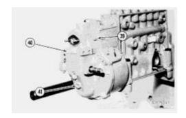
**23.** Remove guide screw (41) from the governor cover. Remove six screws (39) that hold the governor cover to the governor housing.
