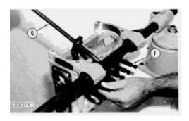
**61.** Use tool (Q) and push down on the lifters and remove tooling (F) from the fuel injection pump housing.
