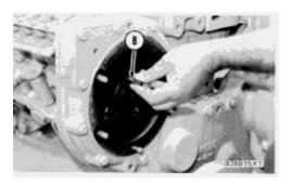
**9.** Install timing pin (8) [tool (C)] through the left top hole (as seen from the front of the engine) in the fuel injection pump gear and through the groove (slot) in the sleeve and into the hole in the adapter of the fuel injection pump. If the timing pin can not be installed at this time, install the timing pin after the fuel injection pump is removed.
