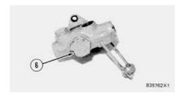
**5.** Remove plug (6), gasket and spring from the housing.
