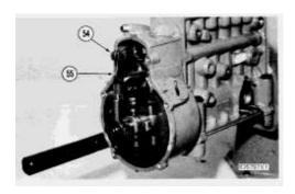
32. Disconnect fulcrum lever (55) from link (54). Use a rubber band to hold link (54) up.
