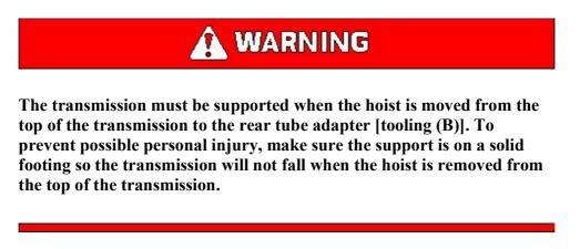
**5.** Put a floor jack or wood blocks in position to support the transmission. Lower the transmission onto the support.
