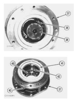
**31.** Use tool (B), and remove retaining ring (39). Remove input shaft (38) from cage (37).
