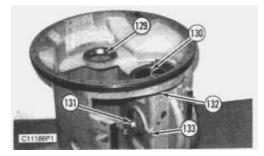
81. Remove bearing cup (129) and the ring under it from the transmission case.
