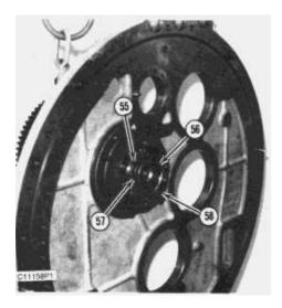
48. Bend lockwasher (57) tab away from the groove in nut (56). Use tool (D), and remove nut (56).
