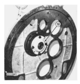
**45.** Install two 5P9736 Link Brackets [part of tooling (C)] to the plate assembly, and attach a hoist. Raise plate assembly (47) to be vertical.
