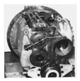
**17.** Remove the two bolts and clips that hold tube assembly (19) in place. Disconnect tube assembly (19) from tube assembly (20), and remove tube assembly (19).
