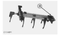
**21.** Remove support assembly (23) from the shifting assembly.
