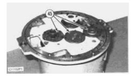
**37.** Remove 18 bolts and three cages (45) from the plate assembly.
