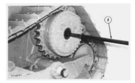
**15.** Use tooling (A) and install the inner and outer axles on both sides. Make sure the first inner axle is not installed too far, or the opposite side inner axle will not go in far enough.
