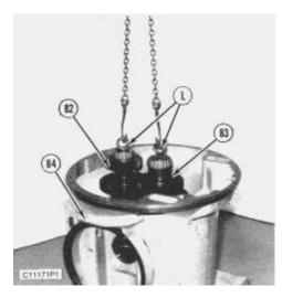
**70.** Install tooling (L) into the end of two gear and shaft assemblies (82) and (83). Attach a hoist as shown. The weight of gear and shaft assembly (82) is **86 kg (190 lb**). The weight of gear and shaft assembly (83) is **75 kg (165 lb**).
