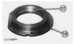
79. Remove bearing cup (127) from cage (123).
