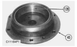
80. Remove bearing cup (128) from cage (45). Cage (45) was removed from shaft (83) in Step 36.
