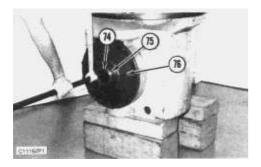
**60.** Bend the tab of lockwasher (75) away from the groove in nut (74). Use took (K), and loosen nut (74) while preventing the bevel gear from rotating, but do not remove it.
