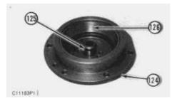
76. Remove seal ring (125) from cage assembly (124).
