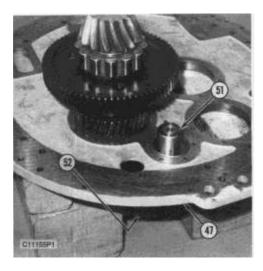
44. Remove six bolts (52) that hold idler shaft (51) to plate assembly (47).
