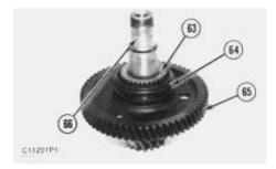
53. Remove collar (64), hub (63) and forward gear assembly (65) from pinion assembly (66).
