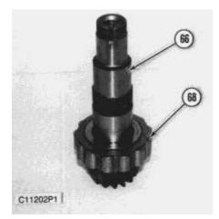
55. Remove bearing (68) from pinion assembly (66).
