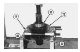
**57.** Use tooling (H) and a press, and remove bearing (71) and input transfer gear (72) from input transfer gear shaft (69).
