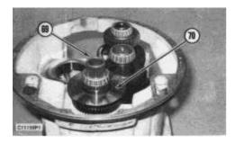
**56.** Remove input transfer gear shaft (69) with brake plate (70), the input transfer gear, and the bearings from the transmission.
