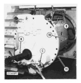
**2.** Install O-ring seal (10) onto the transmission. Install four O-ring seals (9) and (11) onto the transmission and bevel gear case.
