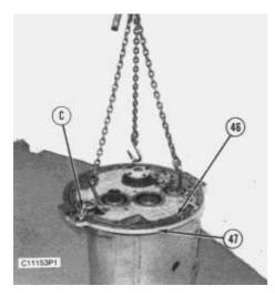
**38.** Install tooling (C) onto plate assembly (47), and attach a hoist.
