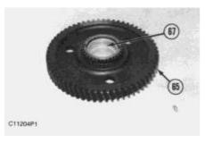
54. Use tooling (G), and remove bearing (67) from forward gear assembly (65).
