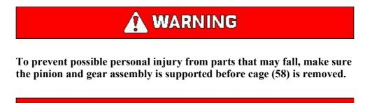
**50.** The weight of the pinion and gear assembly is **24 kg (53 lb)**. Put a nylon strap around the pinion and gear assembly, and attach a hoist. Use two 3/8 **"-16 NC forcing screws** in cage (58), and remove the bearing assembly, the ring, and cage (58). Remove the pinion and gear assembly from the plate assembly.
