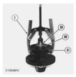
**51.** Use tooling (E) and remove bearing (59), spacer (60), and reverse gear assembly (61) from the pinion assembly.
