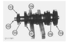
**c.** Remove reverse pinion gear (103), spacer (106), forward pinion gear (107) and sixth gear assembly (104) from countershaft (105).
