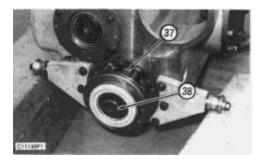
**30.** Remove the six bolts and cage assembly (37) and input shaft (38) from the transmission.
