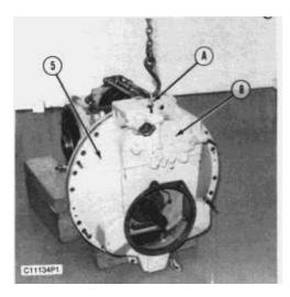
**7.** The weight of cover (5) with clutch control valve (8) installed is **160 kg (350 lb)**. Separate the cover from the transmission a distance of 25.4 mm (1 in), and install tooling (A).
