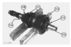
**3.** Use tool (P), and remove retaining ring (115). Remove hub (113) and second gear assembly (112).
