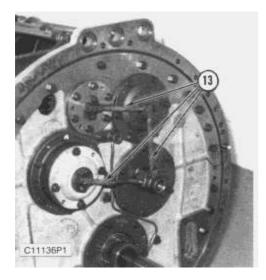
**12.** Remove the eight bolts and three tube assemblies (13).
