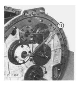
12. Remove the eight bolts and three tube assemblies (13).
