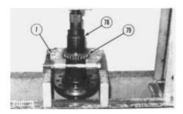
**67.** Use tooling (J) and a press, and remove bearing (79) from bevel gear shaft (78).
