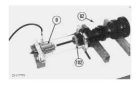
**b.** Install tooling (O), and remove bearing (102) from the countershaft and gear assembly. Use tooling (O), and remove the bearing at the other end of countershaft and gear assembly (82).
