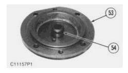
**47.** Remove seal ring (54) from cover assembly (53).
