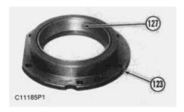
79. Remove bearing cup (127) from cage (123).
