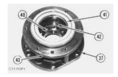
31. Use tool (B), and remove retaining ring (39). Remove input shaft (38) from cage (37).
