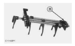
**21.** Remove support assembly (23) from the shifting assembly.
