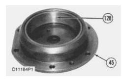
80. Remove bearing cup (128) from cage (45). Cage (45) was removed from shaft (83) in Step 36.
