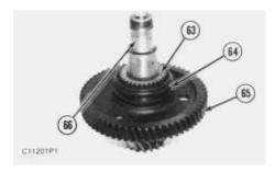
**53.** Remove collar (64), hub (63) and forward gear assembly (65) from pinion assembly (66).
