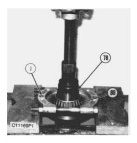
**68.** Turn bevel gear shaft (78) over, and use tooling (J), and remove bearing (80) from bevel gear shaft (78).
