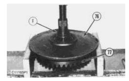
**64.** The weight of bevel gear (77) and shaft is **25 kg (55 lb)**. Use tooling (F) and a press, and remove bevel gear (77) and the shaft from cage (76).
