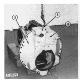
**7.** The weight of cover (5) with clutch control valve (8) installed is **160 kg (350 lb)**. Separate the cover from the transmission a distance of 25.4 mm (1 in), and install tooling (A).
