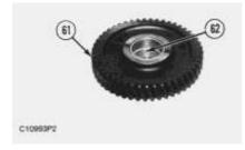
**52.** Use tooling (F), and remove bearing (62) from reverse gear assembly (61).
