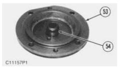
47. Remove seal ring (54) from cover assembly (53).
