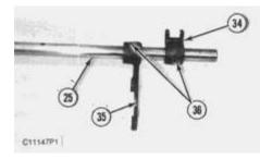
**29.** If necessary, use a hammer and a punch, and remove pins (36). Remove guides (34) and forks (35) from shafts (25).
