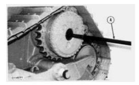
3. Remove the final drive cover and sun gear retainer from the final drive carrier.
