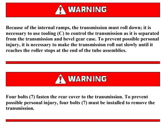
**9.** Remove the 21 bolts that hold the transmission to the transmission and bevel gear case. Four bolts (7) should not be removed because they hold the rear cover to the transmission.
