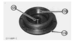
76. Remove seal ring (125) from cage assembly (124).
