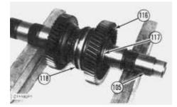
i. Use tool (N), and remove retaining ring (117).
