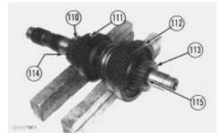
**3.** Use tool (P), and remove retaining ring (115). Remove hub (113) and second gear assembly (112).
