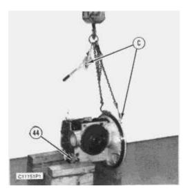
**35.** Install tooling (C), and attach a hoist. The weight of the transmission is **775 kg (1705 lb)**. Raise the transmission, and remove the six bolts and two support assemblies (44) from the transmission.
