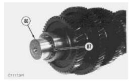
**b.** Use tool (N), and remove retaining ring (87) from input shaft (86).
