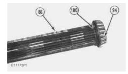
f. If necessary, use tooling (M), and remove bearing (94) from input shaft (86).
