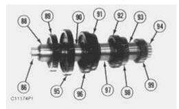
c. Remove spacer (88), input transfer gear (89), and pinion gear (95) from input shaft (86).
