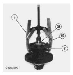
**51.** Use tooling (E) and remove bearing (59), spacer (60), and reverse gear assembly (61) from the pinion assembly.
