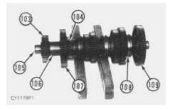
**c.** Remove reverse pinion gear (103), spacer (106), forward pinion gear (107) and sixth gear assembly (104) from countershaft (105).
