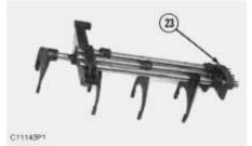
**21.** Remove support assembly (23) from the shifting assembly.
