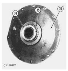
63. Remove nut (74), lockwasher (75) and the washer from the bevel gear shaft and cage (76).
