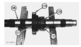
**k.** Use tool (P), and remove retaining ring (120).
