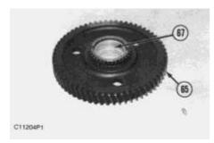
54. Use tooling (G), and remove bearing (67) from forward gear assembly (65).
