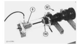
**b.** Install tooling (O), and remove bearing (102) from the countershaft and gear assembly. Use tooling (O), and remove the bearing at the other end of countershaft and gear assembly (82).
