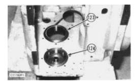
74. Remove the six bolts. Use forcing screws, and remove cage (123) from the transmission case.
