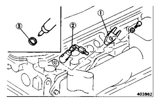
Take off nozzle gland (1), and remove injection nozzle (2) and gasket (3).
