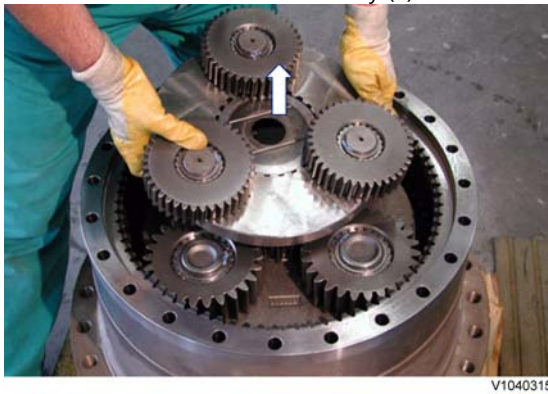
Figure 5 Removal, 1st stage sun gear
