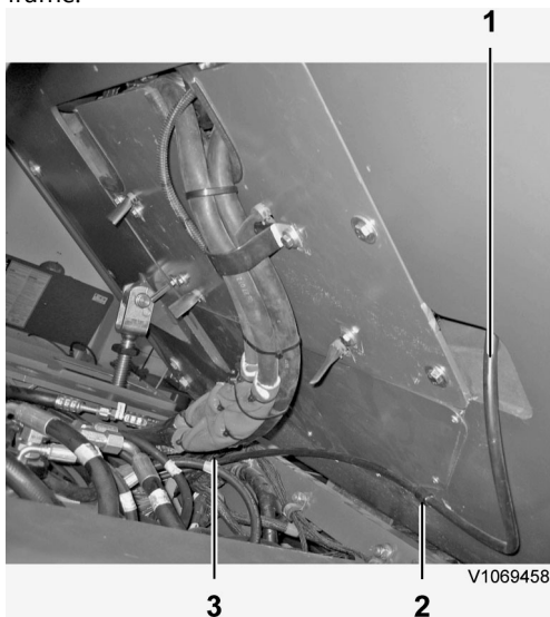
Figure 2 Controller cable routing below the operator's platform
