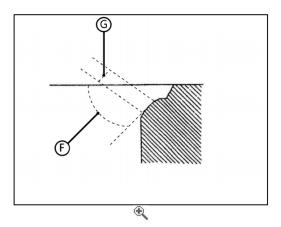
Check the valve face angle (F) and valve seat width (G).
