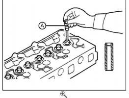
Insert a new valve (3) in the guide (1); make sure the valve slides in the guide freely.
