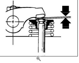
After adjusting the valve clearance on the valves for all cylinders, rotate the crankshaft two or three times and check that the valve clearances are still correct.
