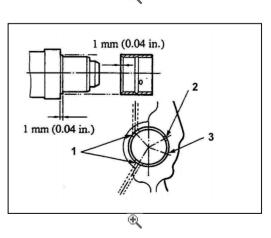
Measure the cam lobe height and base circle as shown in the figure. Subtract the base circle from the lobe height to find the cam lift. If the cam lift
