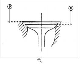
Set the valve refacer at an angle of 45' and grind the valve.
