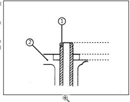
Insert a new valve (3) in the guide (1); make sure the valve slides in the
