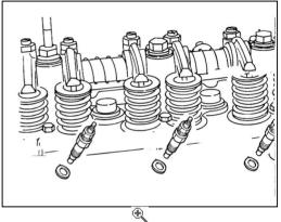
Remove the control rod cover; remove the control spring using pliers, and disconnect the control rod from the injection pump, then remove the a star Q
