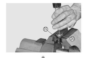
Using a suitable tool, remove bushes (36) from levers control sleeve (8).
