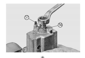
Using a suitable tool, remove guide bush (57).
