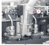
o Tighten the screws (1): 21 Nm.
