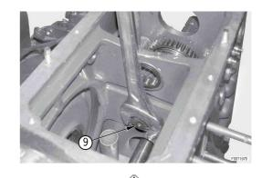
Using suitable tool, partially withdraw PTO output shaft (10).
