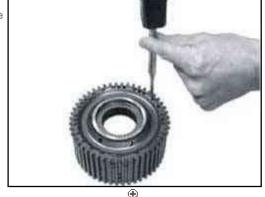
Oil O-ring and then insert it into the annular groove of the disk carrier (see arrow).
