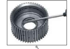
If necessary, disassemble O-ring (fixation of screen sheet, see arrow).
