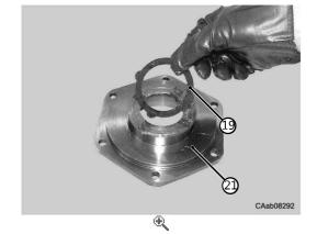
Lubricate a new O-ring (20) and install it in cover (21).
