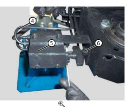
Remove bracket (6) and disconnect front diff. lock pipe (7).
