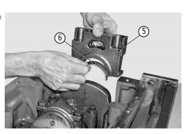
Remove the screws and remove rear main bearing (7) complete with main bearing shell and crankshaft half thrust washers (8).
