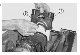
Remove the screws and remove rear main bearing (7) complete with main bearing shell and crankshaft half thrust washers (8).
