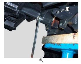
Remove screws (12) on the pipe bracket.
