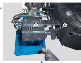
Remove bracket (6) and disconnect front diff. lock pipe (7).
