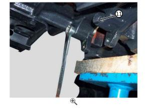
Remove screws (12) on the pipe bracket.
