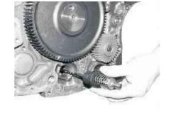
• Fit and tighten the new screw (1): 10 Nm.
