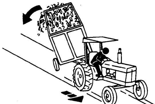
Ensure the load does not exceed the recommended weight ratio. Add ballast to recommended maximum for tractor, lighten the load, or get a heavier towing unit. The tractor must be heavy and powerful enough with adequate braking power for the towed load. Use additional caution when towing loads under adverse surface conditions, when turning, and on inclines.
