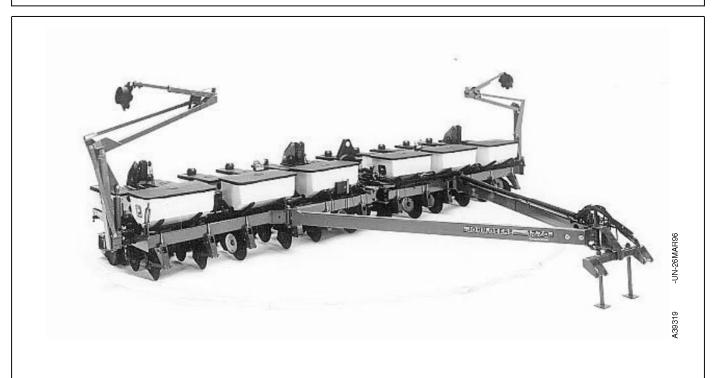
1770 Flex-Fold 12-Row Narrow Drawn MaxEmerge® Plus Planter with VacuMeter Seed Metering System and Dry Fertilizer Attachment
